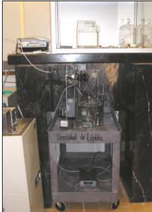
Fig. 2. Hydrostatic weighing system of CENAM. Thermostatic bath implemented by CENAM for this bilateral comparison.
